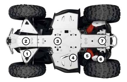
For ultimate durability and strength, all our Aluminum Skid Plates are made with ¾16" (4.5 mm) thick High Strength 5052 H32 Aluminum.
